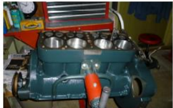
The #8 stud sits right next to the narrow area between #3 and #4 cylinder.
