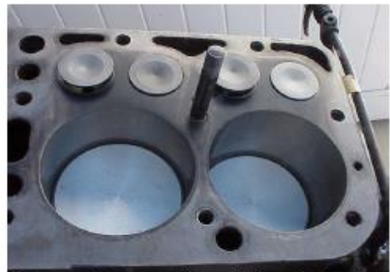
The area between #3 and #4 cylinder is a common place for a blown head gasket. The #8 stud sits right next to the area.
